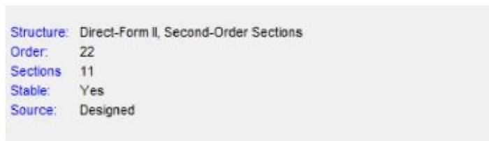
Figure 3.18 Elliptic filter Order and Section count
