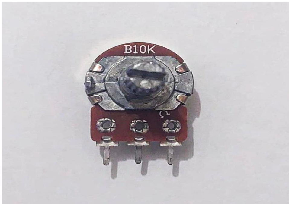
Figure 4.7: Variable resistance that controls the degree of drug
