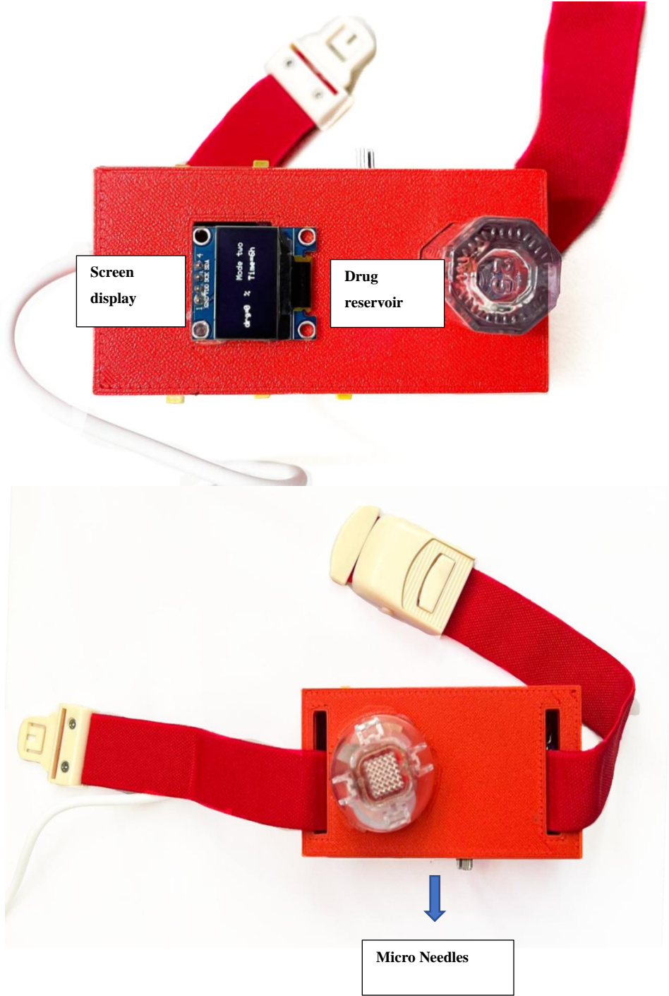
Figure 4.5: Micro Needles for Drug Delivery (Pottom view)
