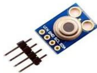
Figure 6: show that the 3temperature sensor mlx90614
