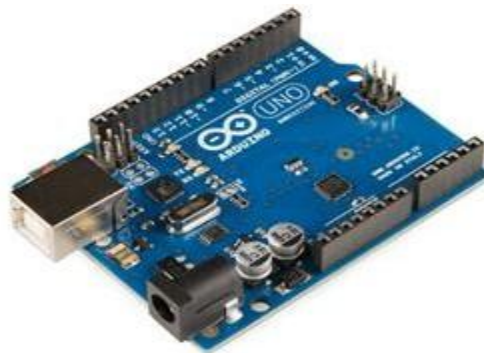
Figure 4: show that the electronic development board of Arduino
