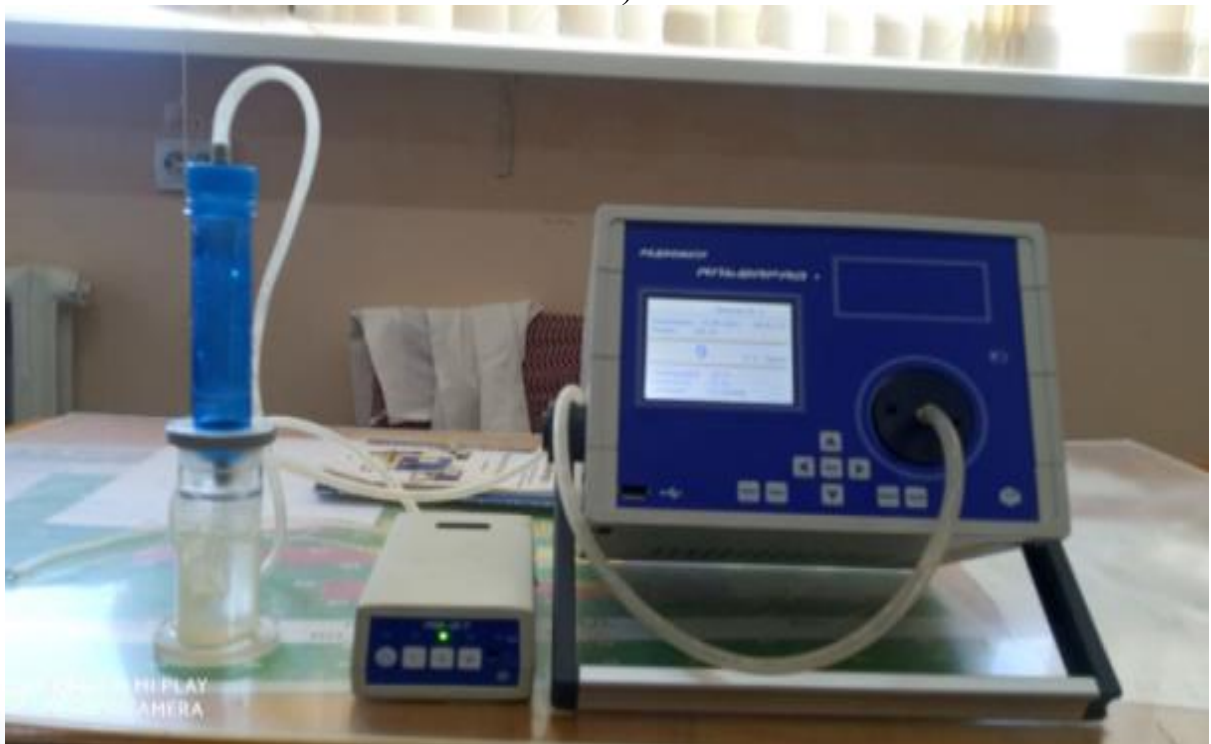
Fig. 3.5 –a-b. The process of measuring the exposure dose rate of radiation radiation factors in the air with the DKS-96 measuring device.
