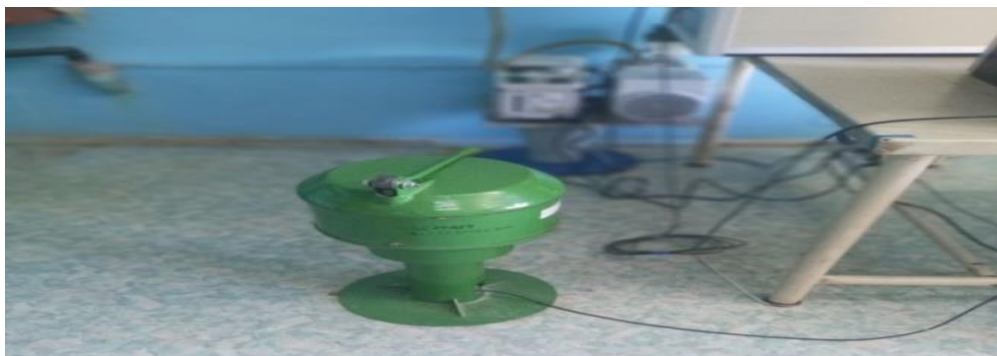
Figure 4.8. The process of measuring crushed soils by the gamma-spectrometric method on the "Progress-gamma" device.
